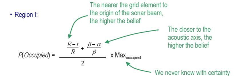
where r is distance to grid element,  $\alpha$  is angle to grid element  $\text{Max}_{\text{occupied}}$  = highest probability possible (e.g., 0.98)
