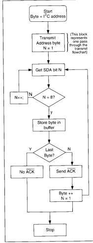
Figure 3: Flowchart for I2C receive procedure.
