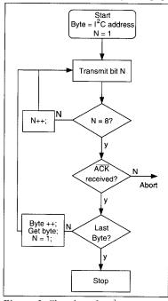
*Figure 2:* Flowchart for I<sup>2</sup>C transmit procedure.
