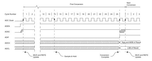
Figure 23-5. ADC Timing Diagram, Single Conversion
