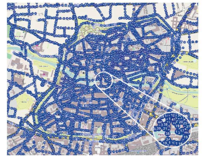
Fig. 1 Example extracted from the Fraunhofer IIS awilo® fingerprinting database in Nuremberg, visualized on an openstreetsmap.org map. Dots indicate fingerprint positions and the amount of detected access points at each position, as depicted in the scale-up
