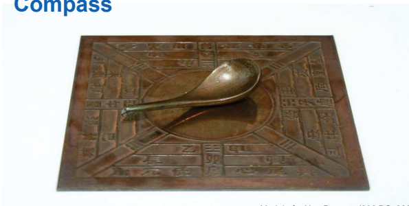
Model of a Han Dynasty (206 BC–220 AD) south-indicating ladle or sinan. It is theorized that the south-pointing spoons of the Han dynasty were magnetized lodestones.
