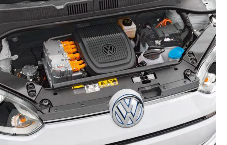
**Wolfsburg, September 2013**. In the new e-up! the compact electric motor (60 kW/82 PS), the lithiumion battery integrated into the floor between the axles and the power electronics form the hub of the car's drive system. The electric motor's power is transferred to the front wheels via a single-speed gearbox. The gearbox and electric motor are both made at Volkswagen components plants.
