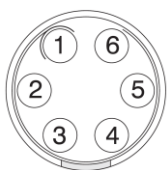
Fig. 8.4: scanCONTROL 27X0 RS422 interface full-duplex (view on solder pin side of connector)
