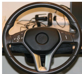
Synaptics demonstration of a steering wheel touchpad with force sensing and haptics.
