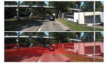
Figure 1: On the left is a LIDAR point cloud (only the data overlapped with the FOV of image are shown, grayscale by height). On the top right is the corresponding image capt by camera. On the bottom right is the result of image and LIDAR point cloud fusion (the well aligned tree trunks).
