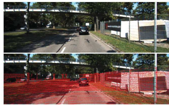
Figure 1: On the left is a LIDAR point cloud (only the data overlapped with the FOV of image are shown, grayscaled by height). On the top right is the corresponding image captured by camera. On the bottom right is the result of image and LIDAR point cloud fusion (the well aligned tree trunks).
