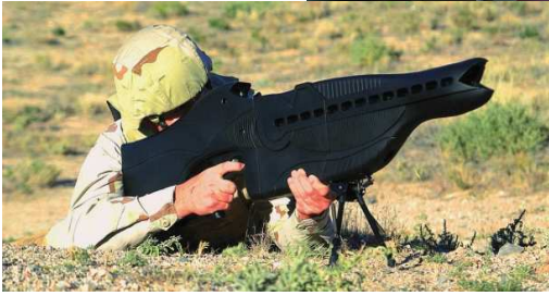
The personnel halting and stimulation response rifle (PHASR) is a prototype non-lethal laser dazzler developed by the Air Force Research Laboratory's. Its purpose is to temporarily disorient and blind a target.
