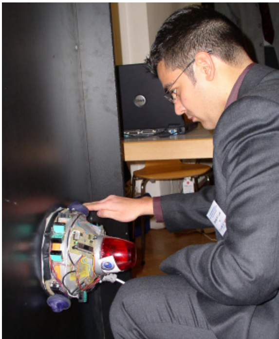
Fig. 6. Robot Alicia (Caltabiano et al., 2004) climbing the wall at the CLAWAR/EURON workshop in Vienna
